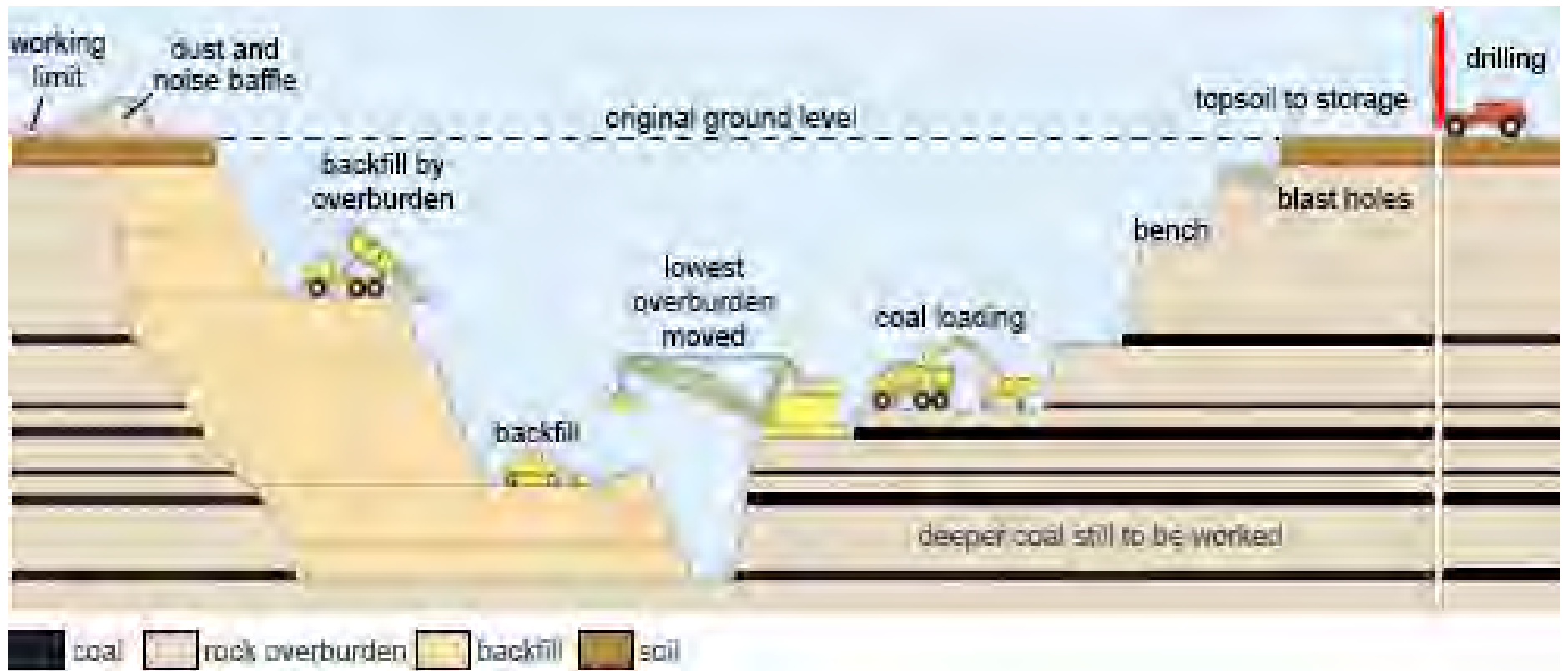
Figure 18 - Surface Mining Diagrammatic Section (Source: The Open University)
